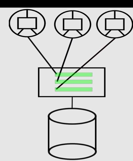
Modern O/S use memorymapped I/O to a kernel buffer. Data transfer via memcpy to userspace.
